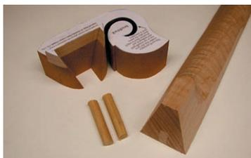
(NOTE: Do not re-shape the flattened side of the neck heel unless you are changing its size to allow the neck to sit lower in the headblock.)
