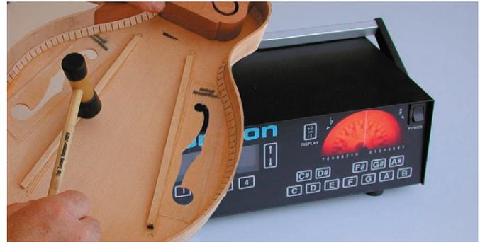
Fig. 2. We recommend the *Peterson AutoStrobe 490*. This tuner features a true mechanical strobe with fast response and great accuracy. The Peterson tuner displays the note in an LCD screen and uses a spinning wheel to display the sharp or flat qualities of the desired note.
