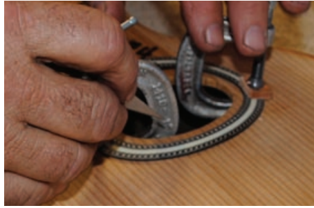
2. Use small wood or leather cauls to protect the rosette and clamp the rosette in place with small C-clamps.
