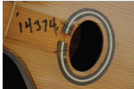
23. Allow to stand for 24 hours and then remove the clamps and wax paper.
