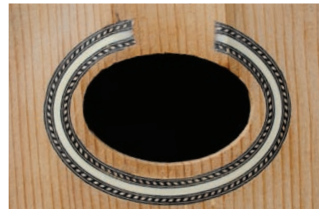
27. The free ends of the rosette that are sanded away will not be visible once the fretboard is in place.
