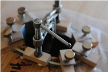
22. Apply some glue under the free ends of the rosette and gently clamp the ends downward (but not all the way).
