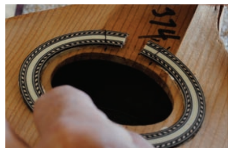
15. Place the rosette into the channel and rotate it to align to the marks you made in Fig 11.
