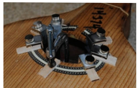
12. Using small clamps and cauls, test-clamp the rosette. Do not clamp the rosette down to the fretboard plane.
