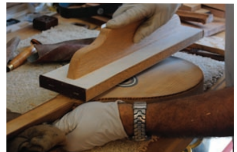
24. Use a flat sanding block to level the protruding ends of the rosette to the fretboard plane.
