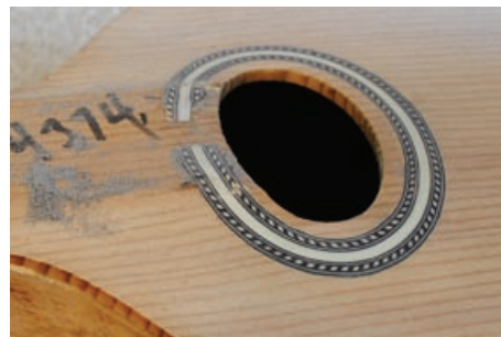
26. Sand the open ends of the rosette flush fretboard plane.
