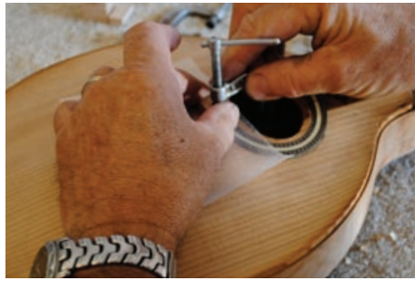
17. Placed cauls on the wax paper and begin to position small C-clamps around the rosette.
