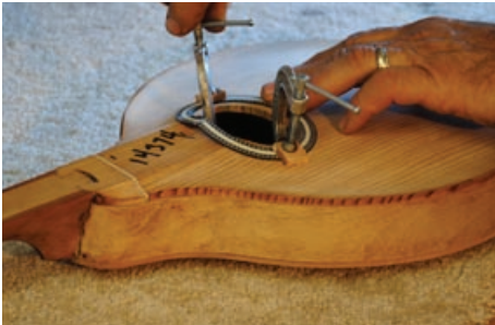
4. Place two more cauls and clamps on the rosette, then remove the first two clamps, and complete the cut.
