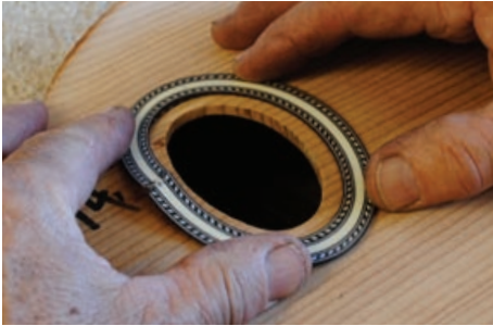
1. With the soundhole cut, position the rosette on the soundboard and align it to the soundhole.
