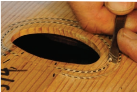
7. Using small chisels or gouges, begin to remove the soundboard wood between the cut lines.
