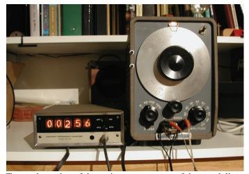
To test the tuning of the various components of the mandolin, a Hewlett Packard<sup>®</sup> Audio Oscillator is con-nected to a speaker and to a frequency counter. The large knob on the oscillator controls the sweep through a range of intervals from 20 to 200. The knob in the lower left corner controls the range intervals such that a setting of "1" equals 20Hz to 200Hz, "10X" equals 200Hz to 2,000Hz, "100X" equals 2,000Hz to 20,000Hz, and "1000X" equals 20,000Hz to 200,000Hz.
