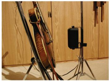
The F5 mandolin was placed on a music stand with the speaker facing it. As the oscillator sweeps through the frequency range, the instrument responds with "sympathetic vibrations" that can be sensed by touch or measured with the aid of a decibelometer.
