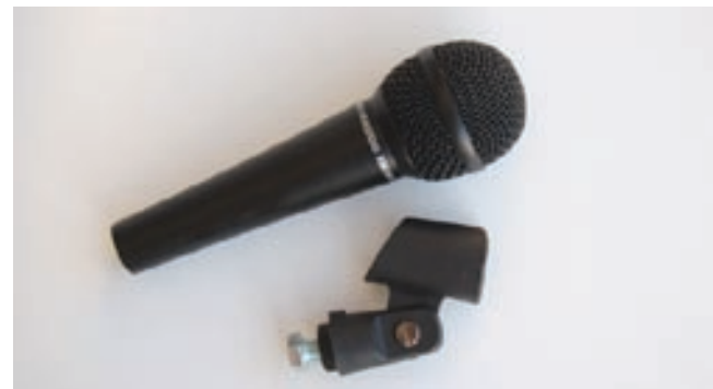
Fig. 9. Tap Tune microphone #826, dynamic microphone modified to be more directional, with slide-in base and mounting screw.
