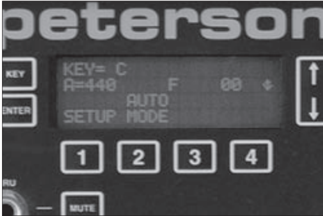
Fig. 5. The four FUNCTION keys, 1 thru 4 control the settings that appear directly above them in the LCD menu screen.
