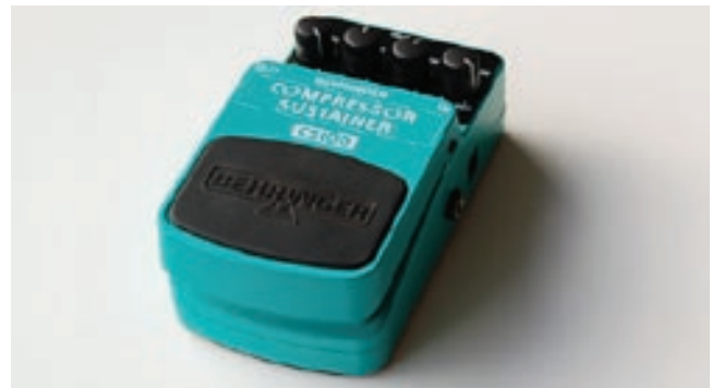
Fig. 8. Compressor, #825, to expand the sustain of tapped notes. Microphone plugs into compressor, compressor plugs into strobetuner.
